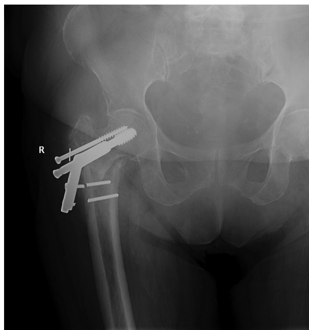
Figure 3. X-ray showing implant breakage (cortical screws) in 2-hole DHS system (from author's personal archive)
